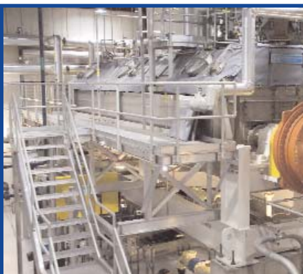
The end process, or sludge drying, for sludges before they are hauled off site. The drier the product is, the less it weighs, and thus, the less it costs to remove.
